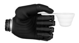
Mouse This grip is used to operate a computer mouse. The hand assumes the position of the mouse. The index finger and the middle finger can be controlled to push left and right buttons respectively.
