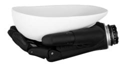
This grip is used for lifting up heavy objects like briefcases, shopping bags and gym equipment. Because of the self-locking nature of Zeus, the fingers have a static grip capacity of 35kgs, allowing you to lift heavy objects with ease. This grip can also be used to provide support when getting up from a seated position.
