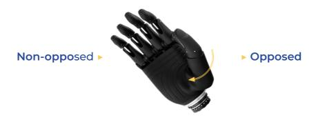
To move the thumb from the opposed to the **non-opposed position**, please hold the thumb at its base with your free hand and push it steadily outwards in a controlled manner.
