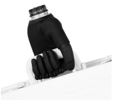
Key This is a commonly used grip for picking up thin flat objects, holding a key or turning a page. The four fingers assume a position to provide a flat platform for the thumb. The thumb can be controlled proportionately to open and close.
