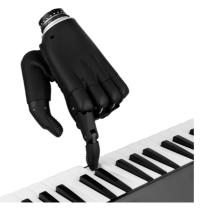
The index finger is active and in a pointing Active position with the rest of the fingers open. This can be used for working on computer Index keyboard, typing.
